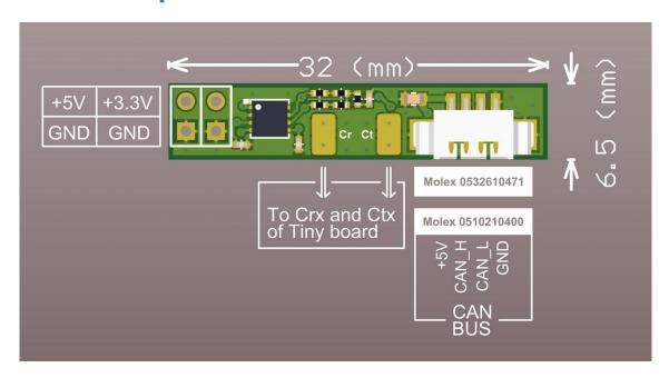
Note. CAN adapter requires 3.3V and 5V supply. Connect the adapter contacts to the corresponding contacts of the main controller. Stable operation of the adapter with 3.3V and 5V supply from other sources is not guaranteed!
